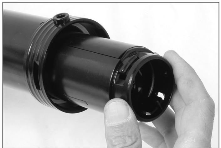
3. With the swirl sleeve fully removed it can either be cleaned or replaced.
