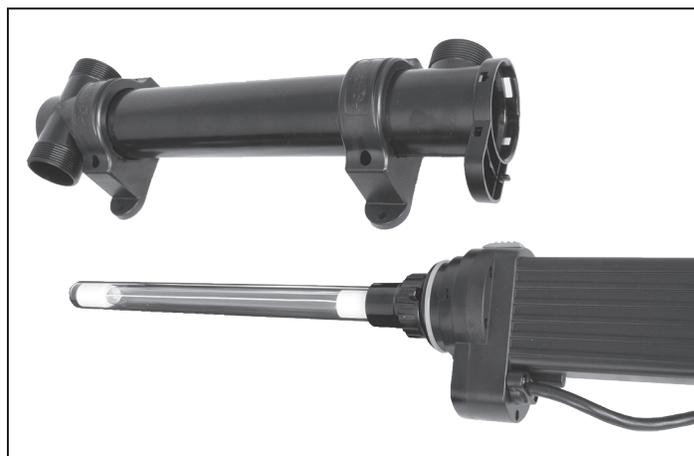
5. If replacing or removing the quartz tube remove the threaded plastic collar at the base of the quartz sleeve and remove the quartz tube.
