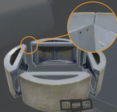
Place the 4 pieces together. Line up the holes on each piece with the corresponding holes and drill in the self tapping screws. Do this for all 8 screws.
