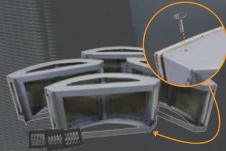
The AnF Round comes shipped as 4 individual pieces. Start by installing the leveling legs into the bottom of the unit. Make sure you screw the bolt in until their is about 1" of clearance.
